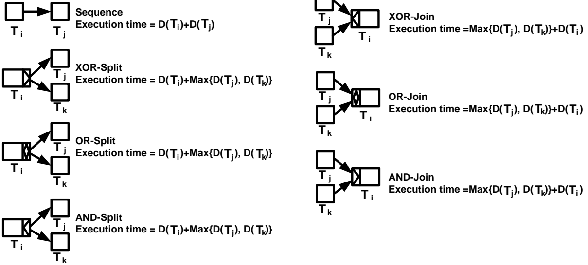
Figure 5. Execution time for different control patterns [8]
