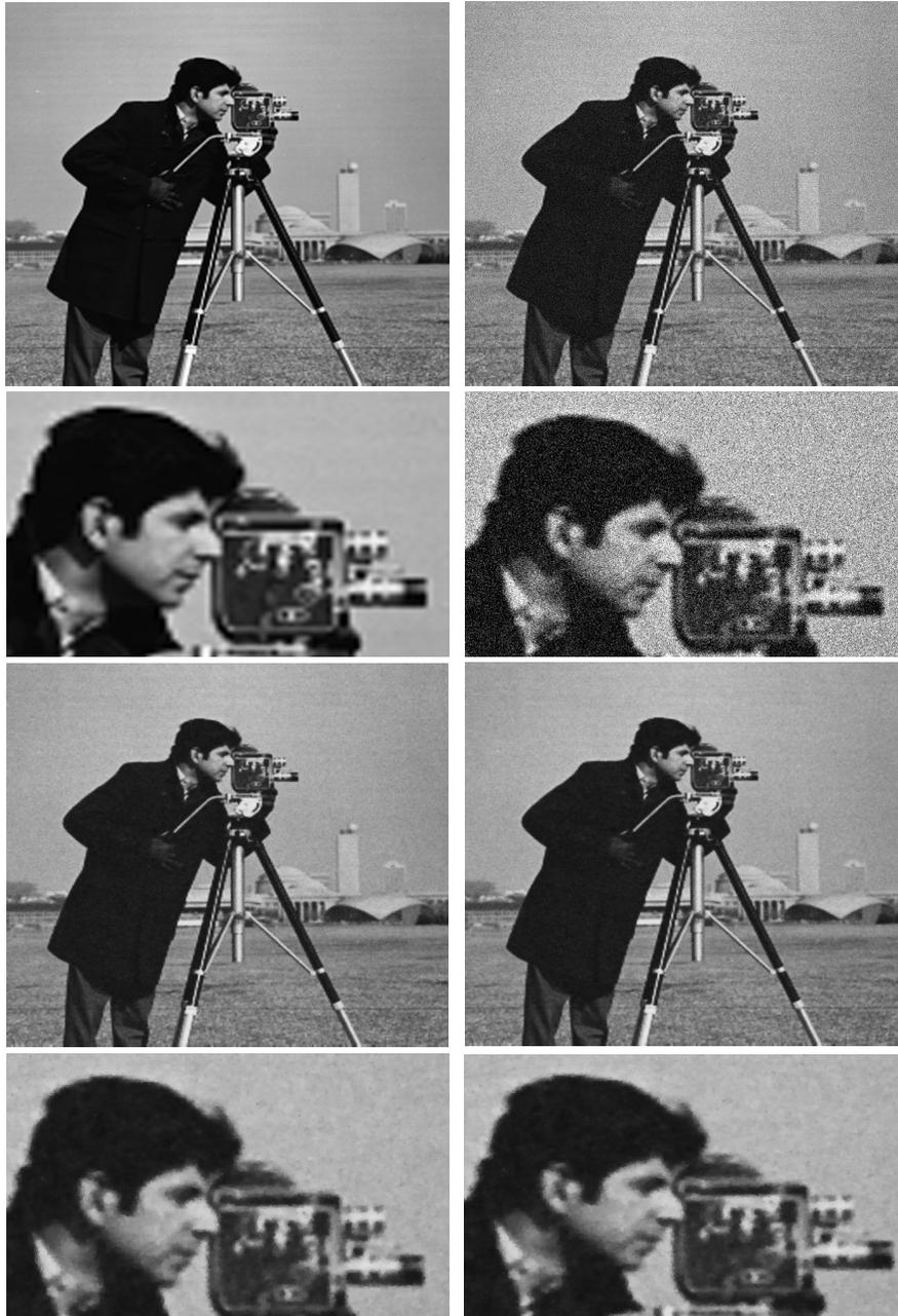
FIGURE 4. A comparison of the results obtained by NiOS and NKS. The first row: the clean image (left), the noisy image with  $\sigma^2 = 0.04$  (right); second row: the local zoom-in of the figures in the first row; third row: the restored images obtained by NiOS (left) and NKS (right); fourth row: the local zoom-in of the figures in the third row. The PSNR of the restored image with NiOS and NKS are 28.536962 and 28.536417, respectively.
