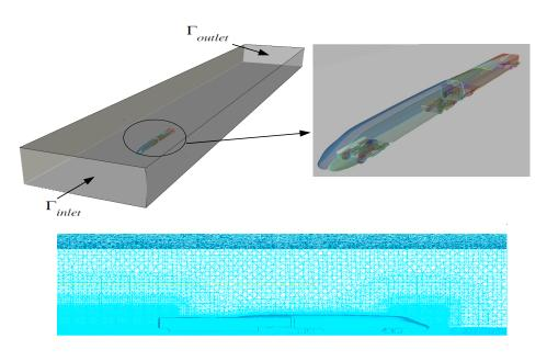
Fig. 4 Model for the simulation of the flow around a high speed train (top) and the mesh around the train (bottom). Here the size of the box (top left) is  $140m \times 23m \times 9m$  and the dimension of the train (top right) is  $19m \times 3m \times 2m$ .
