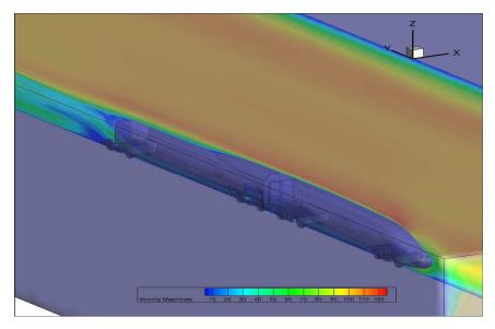
Fig. 5 The velocity distribution around the train at t = 1.0s. Here  $v_{in} = 100m/s$ ,  $\mu = 1.83 \times 10^{-5} pa \cdot s$ ,  $Re = 10^7$ .
