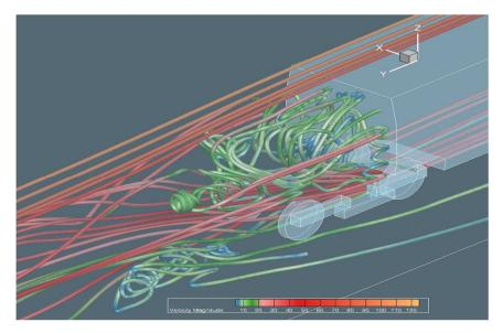
Fig. 7 The stream trace of the flow at the end of the train at t = 1.0s. Here  $v_{in} = 100m/s$ ,  $\mu = 1.83 \times 10^{-5} pa \cdot s$ ,  $Re = 10^{7}$ .
