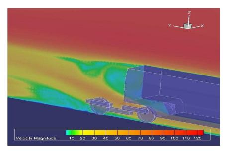
Fig. 6 The velocity distribution at the end of the train at t = 1.0s. Here  $v_{in} = 100m/s$ ,  $\mu = 1.83 \times 10^{-5} pa \cdot s$ ,  $Re = 10^7$ .
