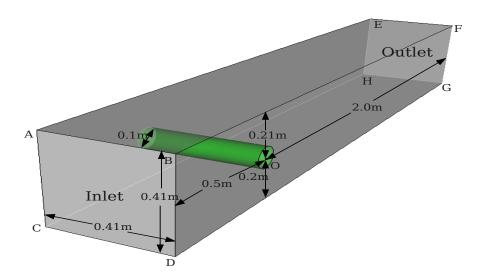
Fig. 1 Flow passing a cylinder in a channel
