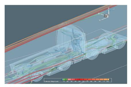
Fig. 8 The stream trace of the flow around the wheels of the train at t = 1.0s. Here  $v_{in} = 100m/s$ ,  $\mu = 1.83 \times 10^{-5} pa \cdot s$ ,  $Re = 10^7$ .
