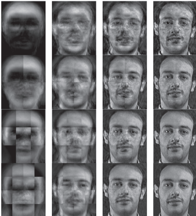
FIGURE 3 The top row shows the reconstructions computed with global principle component analysis (PCA) using 1, 10, 50, 150 eigenmodes; the other three rows of figures show the reconstructions computed with domain decomposed PCA with 2 \times 2 , 3 \times 3 , 4 \times 4 partitions using the same number of eigenmodes, respectively
