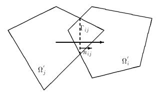
Figure 1: The term  $T_iT_j$  is kept in the Schwarz polynomial only if the flow goes from  $\Omega'_i$  to  $\Omega'_i$ .
