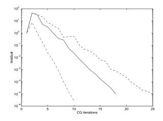
Figure 2: The curves show the iteration history of the additive, multiplicative and the local multiplicative Schwarz preconditioned CG methods. The solid curve represents the local multiplicative Schwarz method, the dashed curve represents the additive Schwarz and the broken curve represents the multiplicative Schwarz method.
