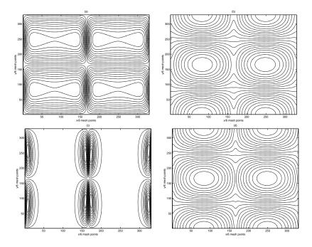
Fig. 4. Contour plots of  $\phi$  (a),  $\psi$  (b), U (c), and F (d). The results are obtained on 1980 × 1980 mesh,  $\Delta t = 1.0\tau_A$ , time  $t = 200\tau_A$ ,  $\eta = 10^{-3}$ ,  $\nu = 10^{-3}$ , implicit time stepping.
