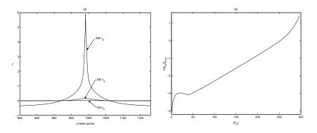
Fig. 7. (a) Time evolution of current density peaks in the reconnection region, 1980 × 1980 mesh,  $\eta = 10^{-3}$ ,  $\nu = 10^{-3}$ ,  $\Delta t = 1.0\tau_A$ , np = 225 with inter-domain overlap  $\delta = 12$ , implicit algorithm. (b) Logarithm of  $|j|_{max}$  as a function of time obtained over all mesh points with the implicit method ( $\Delta t = 1.0\tau_A$ ) on 1980 × 1980 mesh with  $\eta = 10^{-3}$  and  $\nu = 10^{-3}$ , np = 225.
