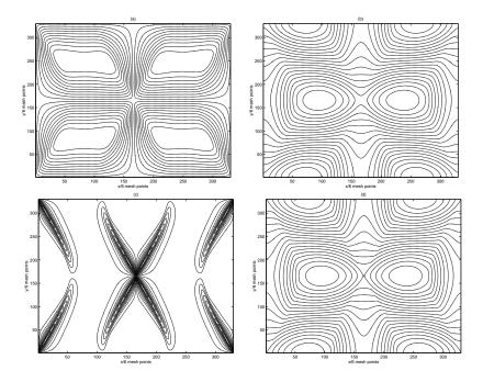
Fig. 5. Contour plots of  $\phi$  (a),  $\psi$  (b), U (c), and F (d). The results are obtained on 1980 × 1980 mesh,  $\Delta t = 1.0\tau_A$ , time  $t = 290\tau_A$ ,  $\eta = 10^{-3}$ ,  $\nu = 10^{-3}$ , implicit time stepping.
