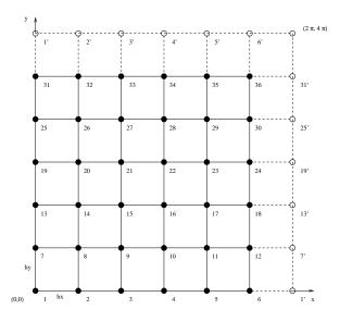
Fig. 1. Rectangular domain  $\Omega = [0, 2\pi) \times [0, 4\pi)$  with doubly periodic boundaries and a sample  $6 \times 6$  mesh. The solid circles indicate genuine mesh points while empty circles denote virtual points that correspond to the boundary mesh points on the opposite side of the domain.
