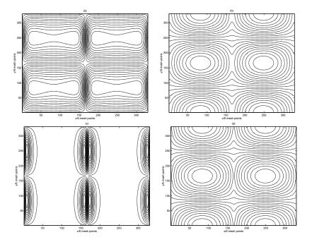
Fig. 3. Contour plots of  $\phi$  (a),  $\psi$  (b), U (c), and F (d). The results are obtained on 1980 × 1980 mesh,  $\Delta t = 1.0\tau_A$ , time  $t = 100\tau_A$ ,  $\eta = 10^{-3}$ ,  $\nu = 10^{-3}$ , implicit time stepping.
