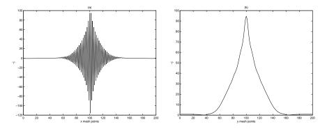
Fig. 8. The highly nonlinear phase of the system's evolution with current density peaks profiles in x direction (a) and y direction (b). The results are obtained on  $200 \times 200$  mesh,  $\eta = 10^{-3}$ ,  $\nu = 10^{-3}$ ,  $\Delta t = 1.0\tau_A$ , np = 1, implicit algorithm.
