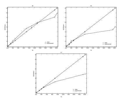
Fig. 12. Speedup curves t(np = 225)/t(np) as compared to the ideal speedup for 1980 × 1980 mesh, LU factorization for all subproblems,  $\Delta t = 1.0\tau_A$ , 10 time steps at times  $t = 100\tau_A$  (a),  $t = 200\tau_A$  (b) and  $t = 280\tau_A$  (c). Physical parameters are:  $\eta = \nu = 10^{-3}$ ,  $d_e = 0.08$  and  $\rho_s = 0.24$ . The straight line in the graphs shows the ideal speedup.
