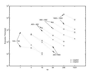
Fig. 10. Execution time comparison between explicit and implicit methods on  $100 \times 100$ ,  $200 \times 200$ ,  $400 \times 400$ ,  $800 \times 800$  and  $1600 \times 1600$  meshes obtained with np = 1, 4, 16, 64, 256, 1024 processors.
