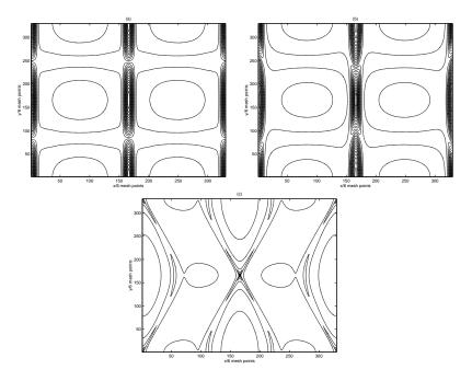
Fig. 6. Contour plots of the current density at  $t = 100\tau_A$  (a),  $t = 200\tau_A$  (b), and  $t = 290\tau_A$  (c). The results are obtained on  $1980 \times 1980$  mesh,  $\Delta t = 1.0\tau_A$ ,  $\eta = 10^{-3}$ ,  $\nu = 10^{-3}$ , implicit time stepping.
