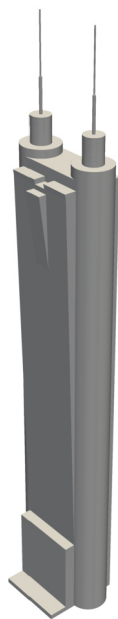
Fig. 7. Geometry of the building Shun Hing Square that was used in the simulation.
