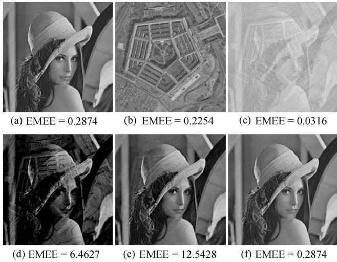
Fig. 9. Demonstration of the case where the parameters are not equal. (a) Original Lena image. (b) Original Pentagon image. (c) Addition of Lena and Pentagon using \gamma(M) = 1026 . (d) Subtraction of (a) from (c) ( k(M) = 256 ). (e) Subtraction of (a) from (c) ( k(M) = 512 ). (f) Subtraction of (a) from (c) ( k(M) = 1026 ). This shows subtraction using the correct value for k(M) .
