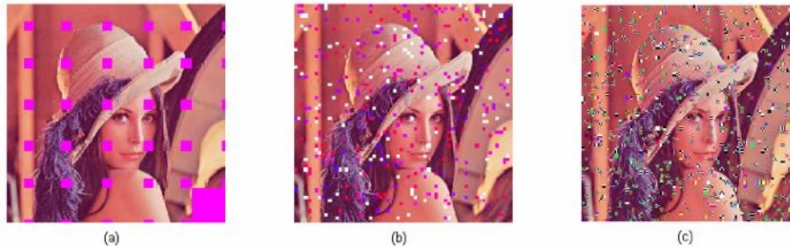
Fig. 7: Reconstructed color images after common attacks in the frequency domain. (a) Reconstructed color image after 1/16 right-bottom cutting attack; (b) Reconstructed color image after 0.1% Gaussian noise attack; (c) Reconstructed color image after 0.1% Salt&pepper noise attack.
