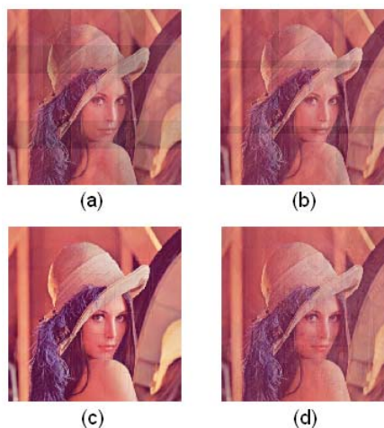
Figure 4. Reconstructed images based on different sequences after a 3x3 Gaussian low pass filter, p=2 . (a) Reconstructed image based on P-Fibonacci sequence; (b) Reconstructed image based on P-Lucas sequence; (c) Reconstructed image based on P-Gray Code; (d) Reconstructed image based on parameter based M-sequence.
