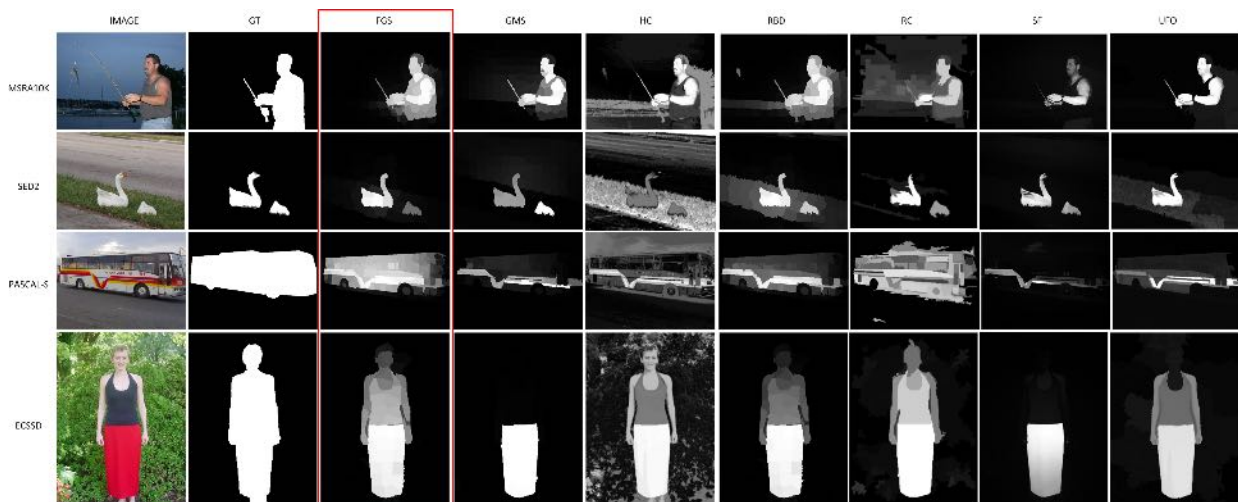
Fig. 5: Visualization of different saliency detection algorithms on different datasets.
