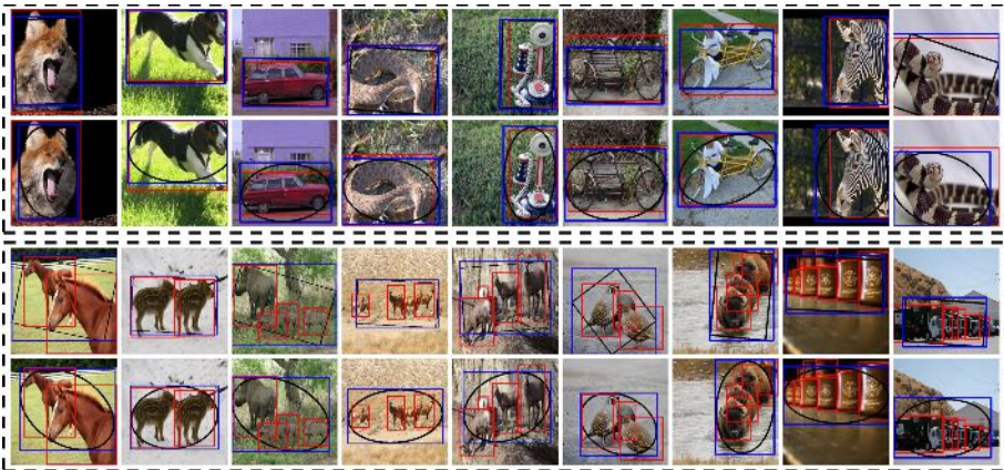
Fig. 7. Localization results on some images from the ILSRC2012 dataset using GC-Net. Top: single object localization. Bottom: multiple object localization. GC-Net tends to predict a bbox that contains all target objects. Ground truth bboxes are in red, predictions are in blue. Rotated rectangles and ellipses are in black, which induced the predicted bboxes.
