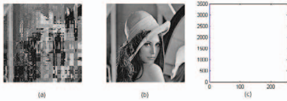
Fig. 5. Grayscale image Encryption with n=2, p=2 for GPGC decomposition and n=3, p=1 for encryption. (a) Encrypted image; (b) Reconstructed image; (c) Histogram of the difference between reconstructed grayscale image and original grayscale image.
