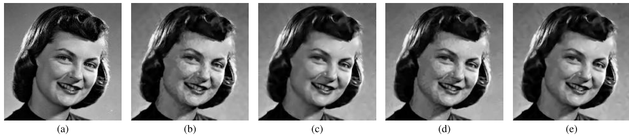
Fig. 9. Denoised results of the girlface image with SNR = 1 : (a) clean image; (b) NL-Bayes; (c) DDID; (d) BM3D; (e) MUD-NLAM-WS.
