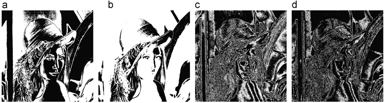
Fig. 1. Image bitplane decomposition of the grayscale Lena image using different methods. (a)–(d) show the 6th bitplane decomposed by the (a) BBD, (b) GCBD, (c) TFPBD with p=1 , and (d) TFPBD with p=2 .
