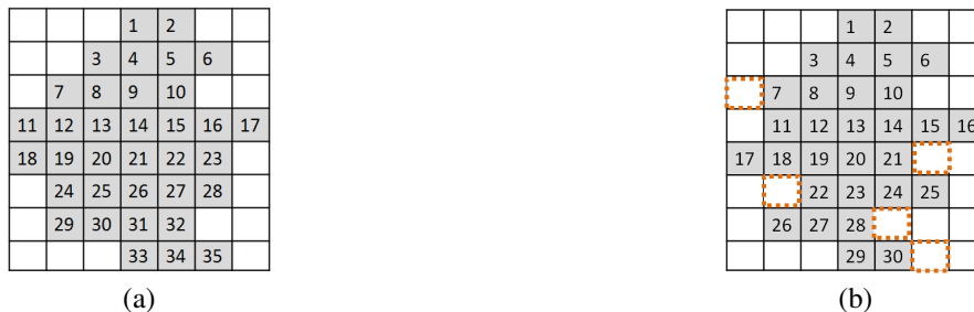
Figure 3. Illustration of embedding messages in an object image. (a) 35 foreground pixels; (b) 30 foreground pixels with several pixels discarded during messages embedding.
