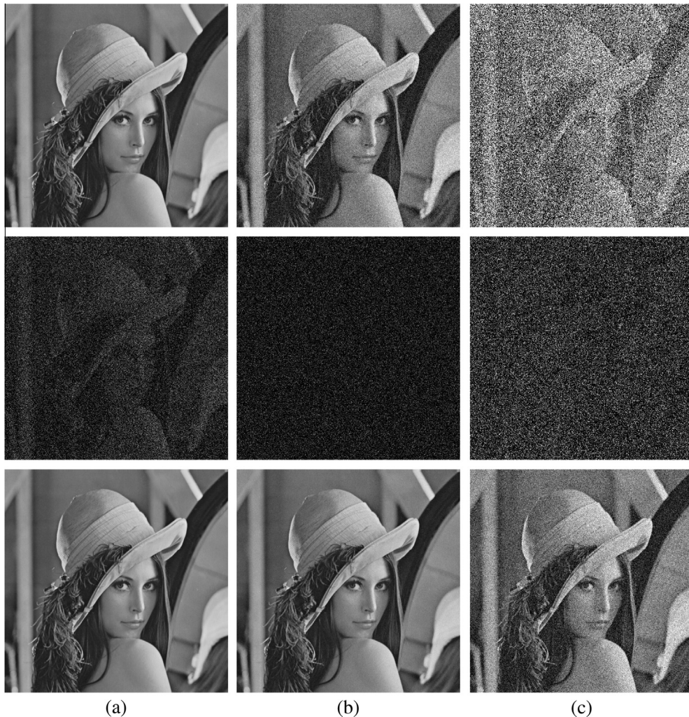
Fig. 9. Noise attack to different image encryption algorithms. The first, second and third rows show the recovered images by the Tao's algorithm [23], Wang's algorithm [27] and MSIEA, from their encrypted images with the noise strengths of (a) 10 dB, (b) 30 dB, and (c) 50 dB, respectively.
