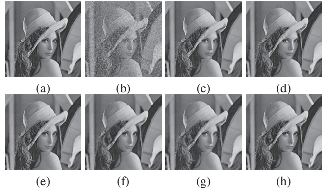
Fig. 1: 'lena' image with 40% random-valued impulse noise restored by different methods. (a)-(b) are the original and corrupted images; (c)-(h) are the restored images by different methods. (c) Luo-iterative method; (d) DWM; (e) CEF; (f) SDOOD; (g) SBF; (h) proposed method. Please zoom into pdf file for a detailed view.
